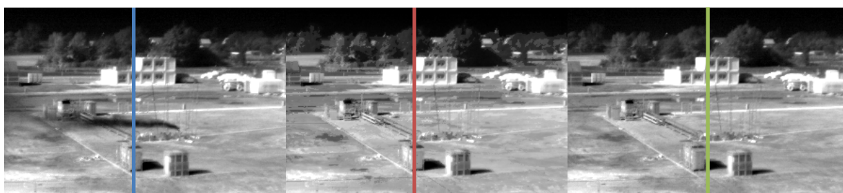
Figure 3-1: Acquired data with gas (left), reconstructed reference (centre), acquired data with gas (right); all at 1303 \text{cm}^{-1}
